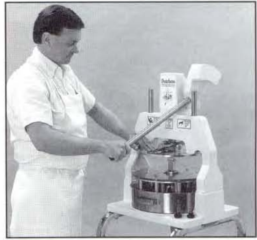
Figure 2: Depress Trip Lever and hold, while pulling Handle down, causing Head Assembly to separate from Trip Lever Plate . . .
