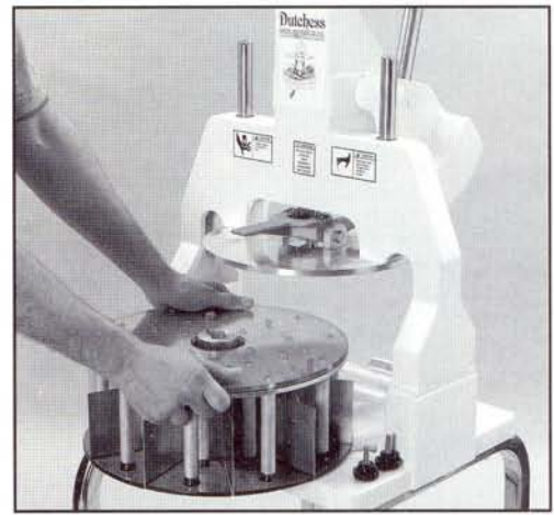
Figure 4: Return Handle to upper position, and remove Head Assembly for cleaning or interchange with Optional Head Assembly.
