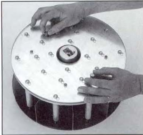
Figure 5: If you wish to disassemble completely, place Head Assembly onto Bench, loosen both Knurled Knobs completely, and lift off Cover Plate . . .
